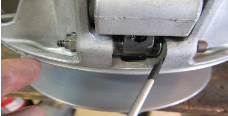
**\*\*Install Thrust Washers-** When installing the Dalton Quick Adjust flyweight, it is **important** to install the supplied thrust washers. One on each side of each flyweight. These Flyweights were designed to be used with these washers. These steel washers offer better, more accurate flyweight movement, and improve durability.
